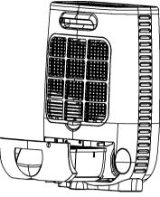
When the water container is full: An alarm signal will sound The Empty Tank LED will flash 🇹 The dehumidifier will stop automatically. Empty the water container and replace it in the correct position. The dehumidifier will start to work again.
